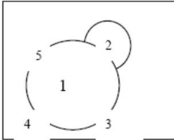
Draw a circle around the sensor's outer edge of 2701 and take readings in the center (1) and at 2 o'clock, 5 o'clock, 8 o'clock and 11 o'clock positions. After reading number 5 is complete, calculate the average of the 5 readings. Press key <1> to save the data after the measurement is completed.
