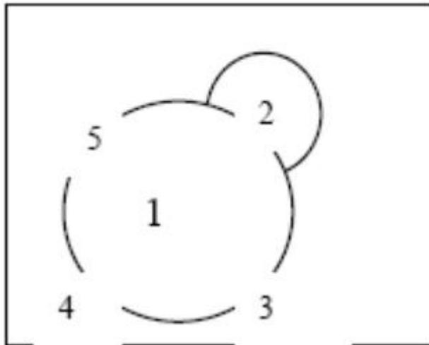
Draw a circle around the sensor's outer edge of 2701 and take readings in the center (1) and at 2 o'clock, 5 o'clock, 8 o'clock and 11 o'clock positions. After reading number 5 is complete, calculate the average of the 5 readings.
